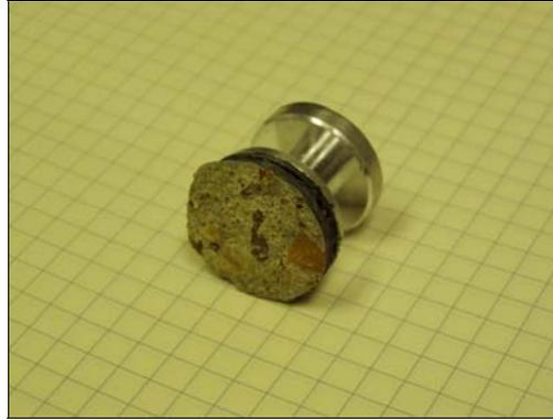
**Figure 6:** Photograph of dolly showing cohesive failure of the concrete substrate
